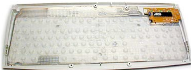
This keyboard uses rubber dome switches.
